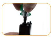
Overfill slightly. Reinstall reference junction cap and tighten until it touches sensor body.
