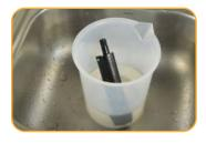
Soak the sensor for two hours in calibration standard. Use at least 140 mg/L solution, or the solution matching your highest calibration point, whichever is greater.
