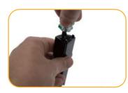
Remove sensor from sonde and unscrew reference junction.
