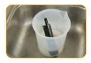
Soak sensor for a minimum of two hours in 355 mg/L chloride standard or the highest standard you plan to use during calibration.
